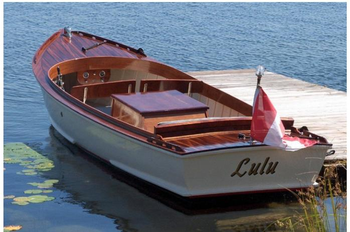
**1922 GEORGIAN BAY ANTIQUE LAUNCH 17'.** Unknown builder. Owner says, "This charming, 1922 launch is powered by a Buchanan Junior 25 hp engine. LULU underwent a complete restoration last year, (2010). Hardware was re-plated and the Buchanan engine was rebuilt. LULU features a cypress wood hull and new sapele wood decks, covering boards and engine box. A custom trailer is... *(continued on page 6.)*
